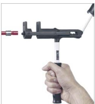
6. Bring tool into starting position and remove expanded pipe. (Open movable lever completely).
