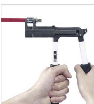
8. Attach tool completely to the joint.
