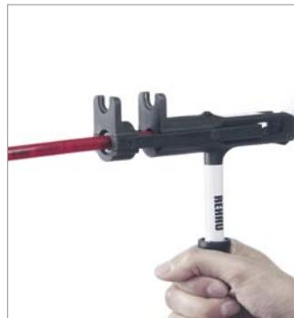
4. Slide pipe through the compression sleeve into the tool up to the stop.
