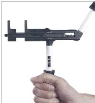
2. Bring tool into starting position. Open movable lever completely ( $\geq 50^\circ$ ).
