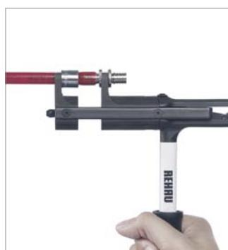
7. Insert fitting into pipe up to the stop. After a brief period the fitting will sit tightly in the pipe (memory effect).
